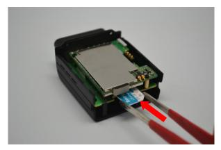
Insert the card with contact on bottom into the slot and push it as far as it will go.
