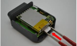
Insert the card with contact on bottom into the slot and push it as far as it will go.
