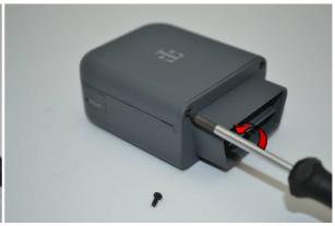
Use slotted screwdriver to pop-out the top cover on both side.
