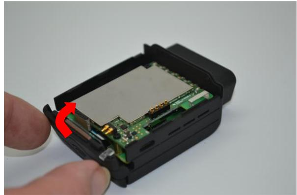
Third, insert the top cover beginning with the back and push on top to clip-on the top cover
