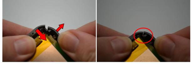
Third, insert the top cover beginning with the back and push on top to clip-on the top cover
