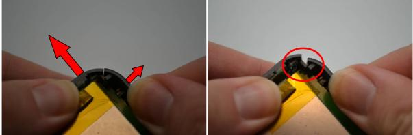
Pull the back cover on the rear and remove the back cover.
