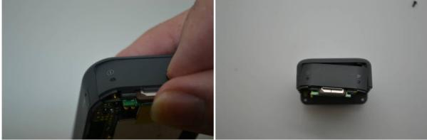
Second, Move apart the side of the device and push the back cover on the spot
