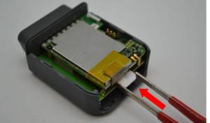
Insert the card with contact on bottom into the slot and push it as far as it will go.
