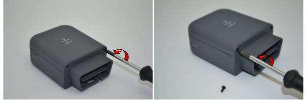
Use slotted screwdriver to pop-out the top cover on both side.
