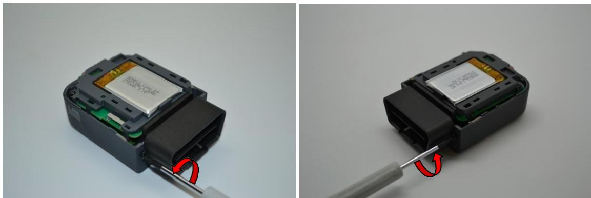
Remove the screw located on the PCB at the bottom of the device using T6 Torx screwdriver
