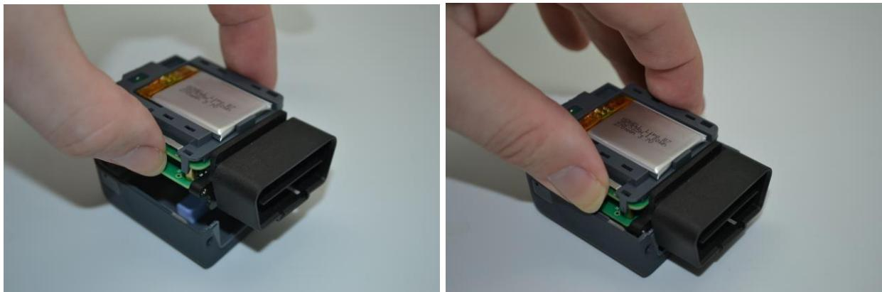
Once inserted, push the main part into the back cover until you hear two "clac"
