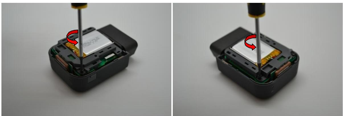
Move apart the side of the device first and then pull the OBD connector out of the body.
