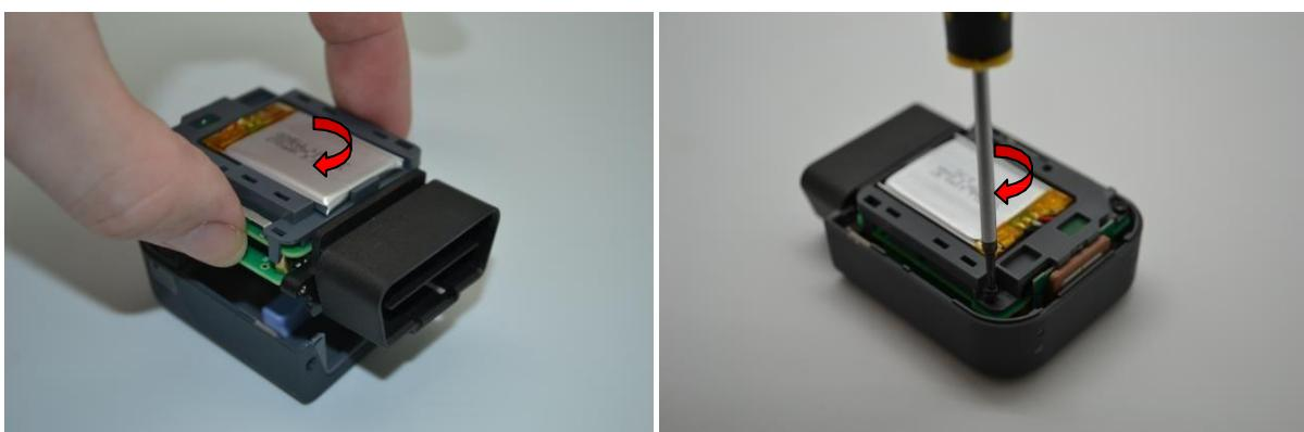
Place the screw on each side of the OBD connector to fix it to the body using T4 Torx screwdriver.
